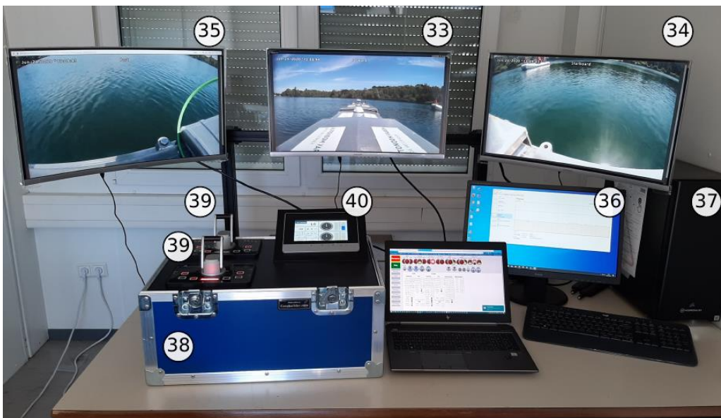
Figure 28: Shore control centre to control Cogge while looking at the available video streams and a real-time overview of useful (sensor) data
