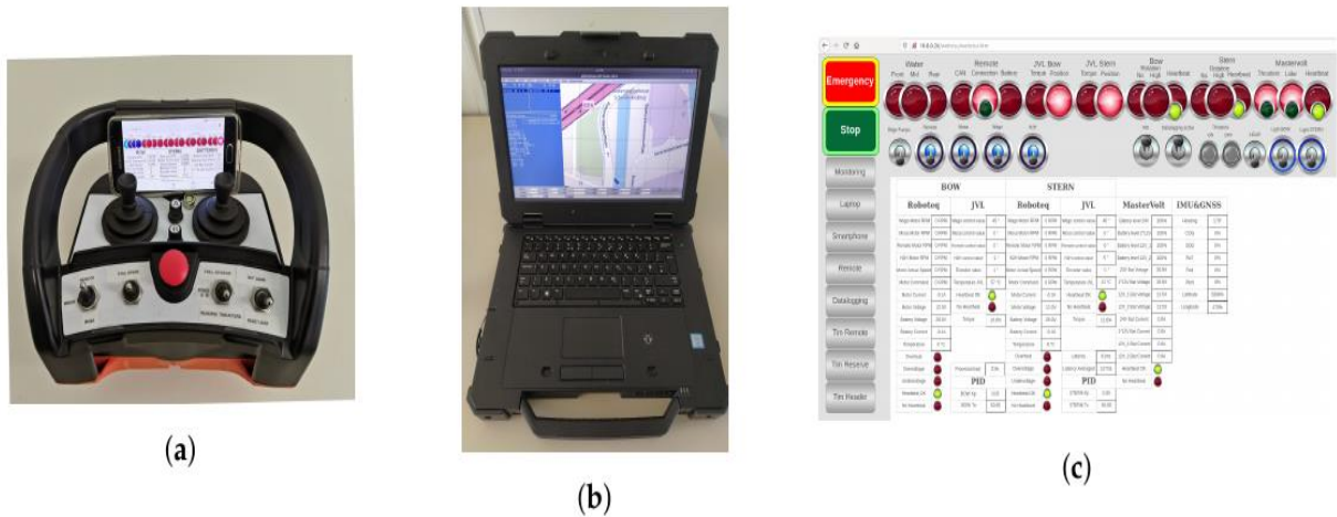
Figure 29: Additional shore-side control components for Cogge: (a) wearable remote controller with web-interface, (b) rugged computer (R-PC) running MOOS-IvP, and (c) an additional laptop monitoring the PLC web-interface
