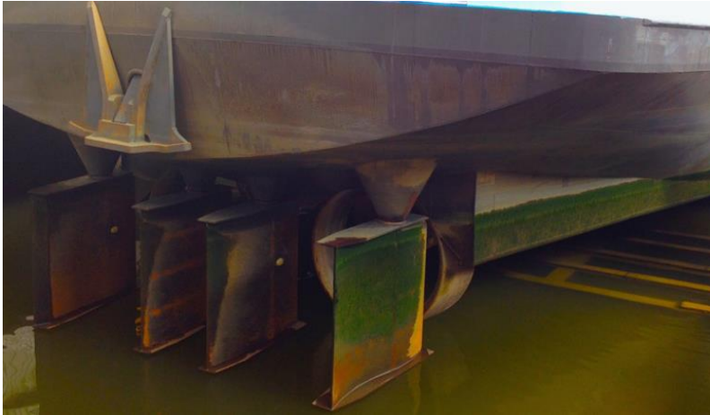
Figure 10: Picture of a typical propeller-rudder configuration consisting of 2 propellers, each with their corresponding rudder. Picture adapted from [6]
