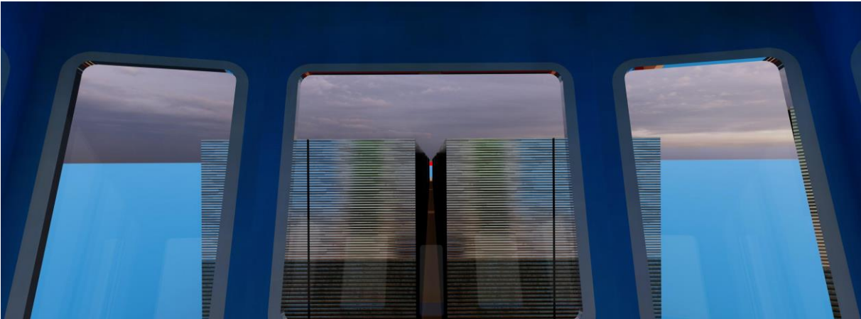
Figure 24: Pusher type 1 with barge 007 IW-NET NEWS Evolution long – 2 layers of 45' high-cube containers 100 % full
