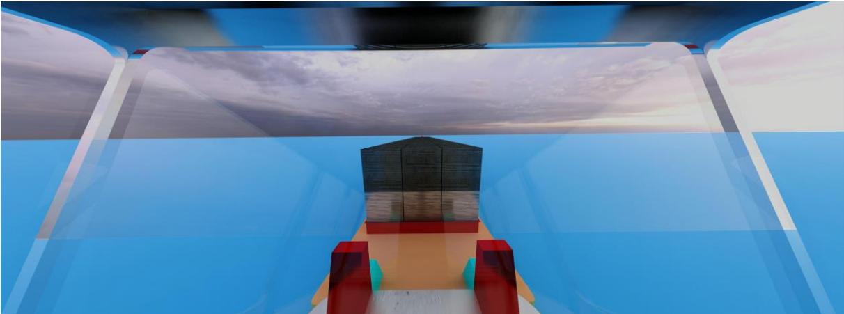
Figure 18: Pusher type 2 with barge 003 IW-NET 3 units abreast – 3 layers of 45’ high-cube containers 100 % full
