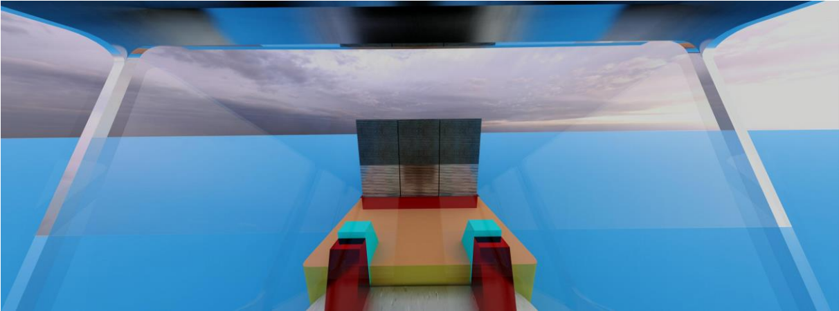
Figure 17: Pusher type 2 with barge 003 IW-NET 3 units abreast – 3 layers of empty 45’ high-cube containers
