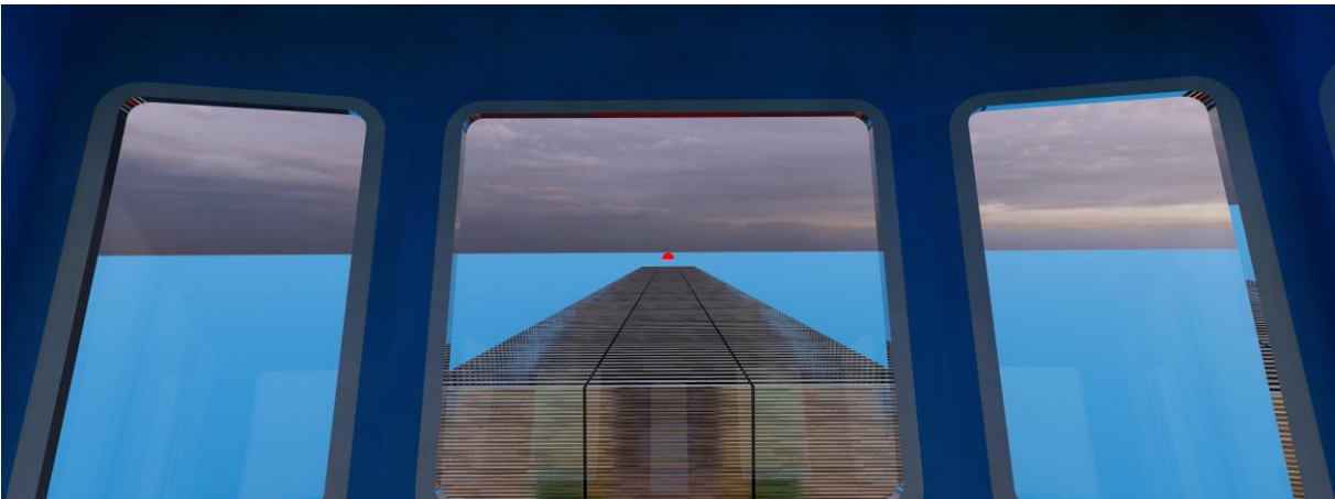
Figure 12: Pusher type 1 with barge 003 IW-NET 3 units abreast – 2 layers of 45’ high-cube containers 100 % full
