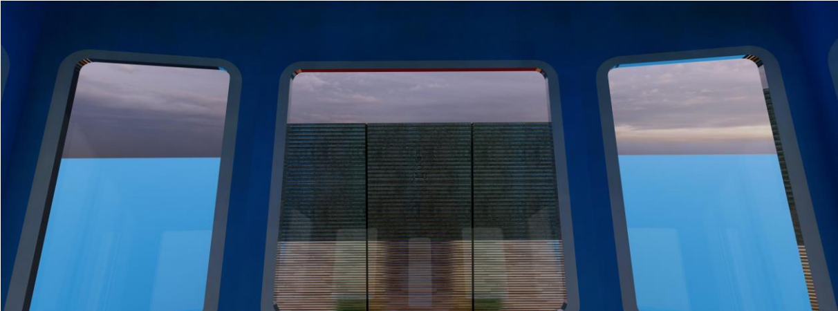
Figure 16: Pusher type 1 with barge 003 IW-NET 3 units abreast – 3 layers of 45’ high-cube containers 100 % full
