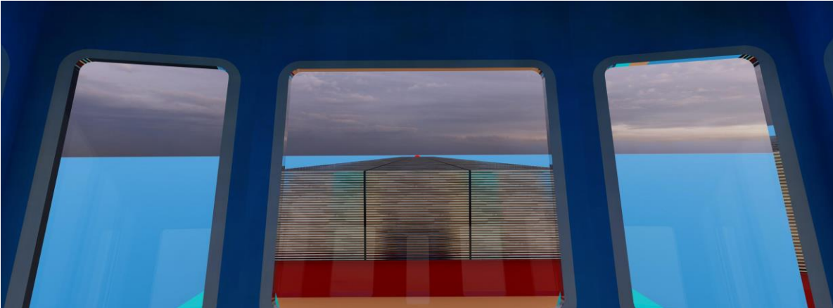
Figure 11: Pusher type 1 with barge 003 IW-NET 3 units abreast – 2 layers of empty 45’ high-cube containers
